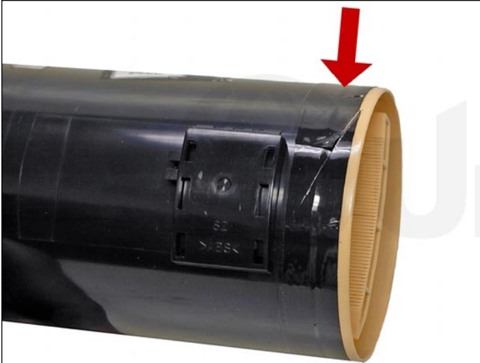
1. Remove the tape from the colored end cap.
