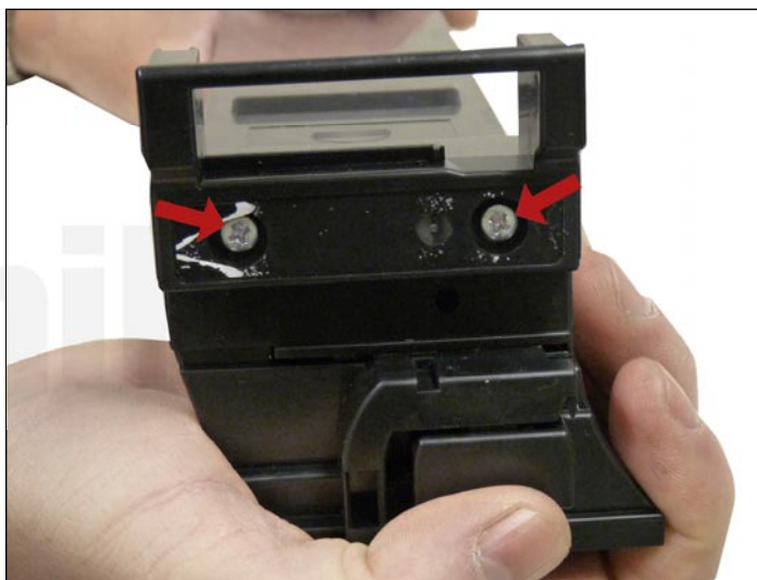
2. Remove the two screws.
