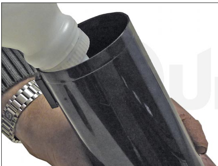
3. Vacuum the tube clean and fill with new toner for use in Phaser 7760.
