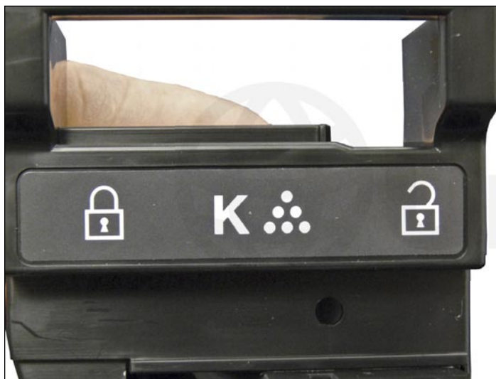
1. Peel the label off the end cap.
